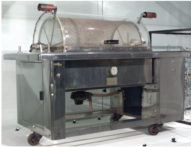
Figure 1.1 Artificial kidney machine (Kolff-Brigham), France, 1955. Source: With kind permission from Science and Society Picture Library.
